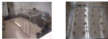
Figure 1. Plexiglas enclosures used to evaluate effects of ultrasound on P. interpunctella reproduction.
