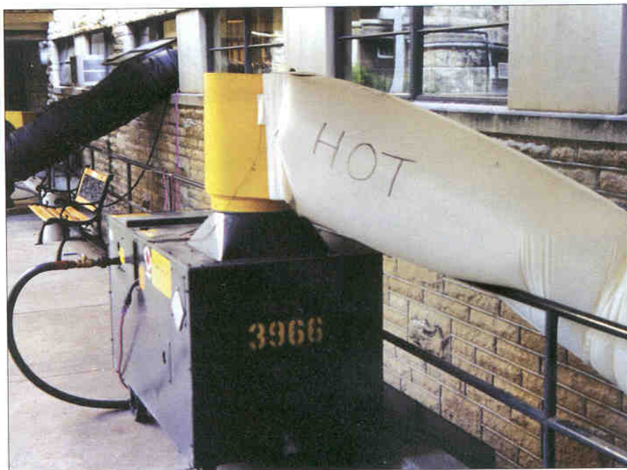
Heat treatments like the TEMP-AIR® Thermal Remediation process, pictured above, that was used to kill insects in the Kansas State University pilot feed mill in August during the heat treatment workshop, are popular alternatives to methyl bromide fumigation.
