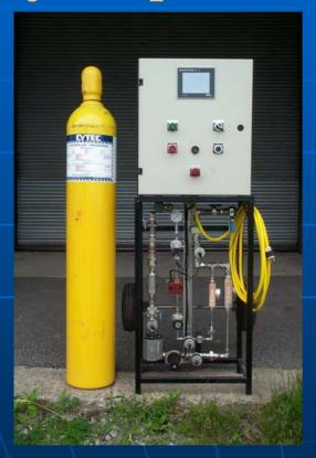
Produces 2% PH<sub>3</sub> Blend PH<sub>3</sub> & Air Blender
