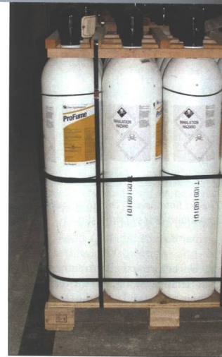
Cylinders of sulfuryl fluoride gas (ProFume®) used in treatments to control insects in Canadian mills.
