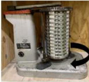
Figure 6. Tyler RoTap sieve shaker with 13-sieve stack
