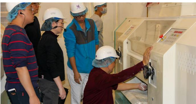
*IAOM-KSU Advanced Milling participants make adjustments to reduction rolls for a starch damage exercise.*
