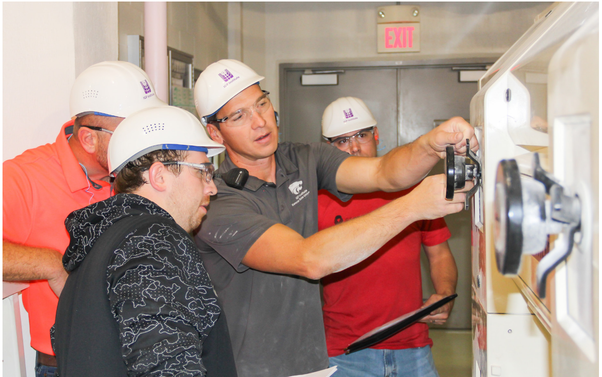
IGP Institute Flour Milling and Grain Processing Curriculum Manager, Shawn Thiele (center), assists participants from the IGP–KSU Advanced Milling course with adjustments to the roll stands in the Hal Ross Flour Mill as part of a hands-on session focused on optimal break release to improve the milling process.
