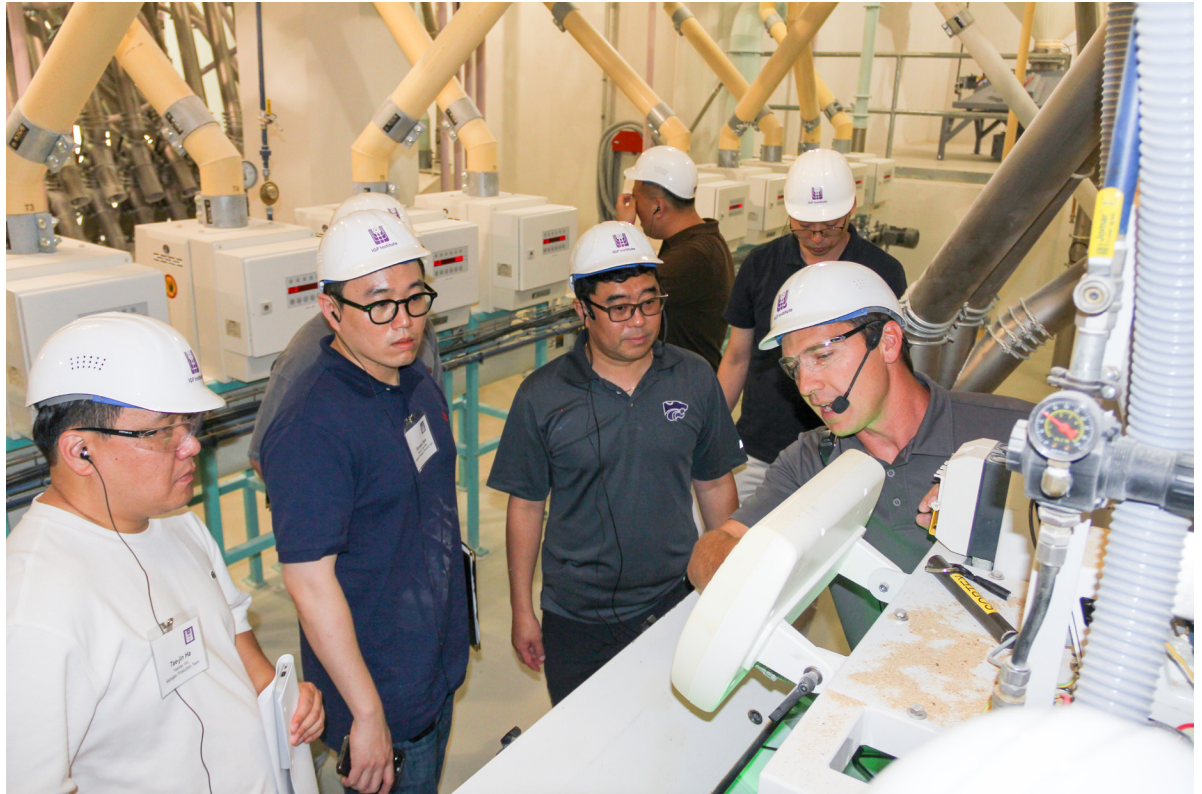
Course instructor, Shawn Thiele, explains the operation of the Sortex optical sorter used to remove discolored and imperfect kernels of wheat before the milling process to participants from the U.S. Wheat Associates/IGP Institute Advanced Milling for South Korea course during an exercise in the Hal Ross Flour Mill.
