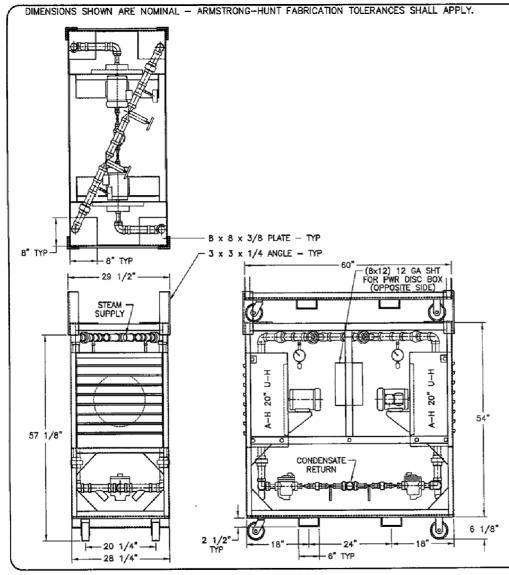
Double Heater Package with Prepiped Temp. Control and Drainage (with Stackable Storage Option)
