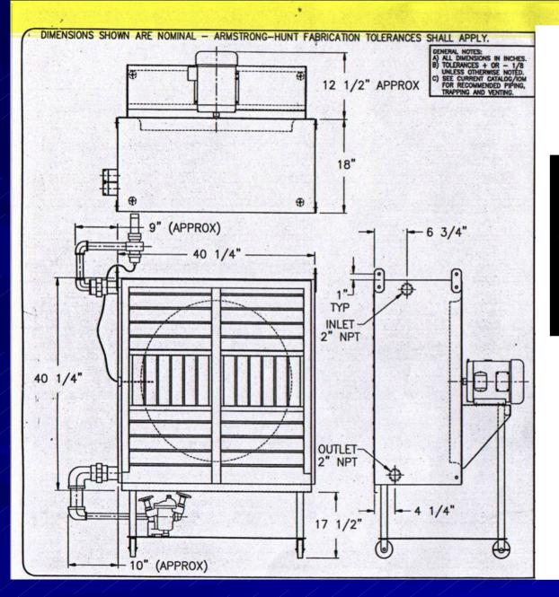
Single Portable with PREPIPED Temp. Controller and Condensate Drainage
