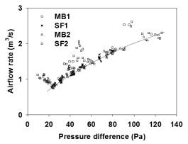
Figure 2 Results of the pressurization tests.
