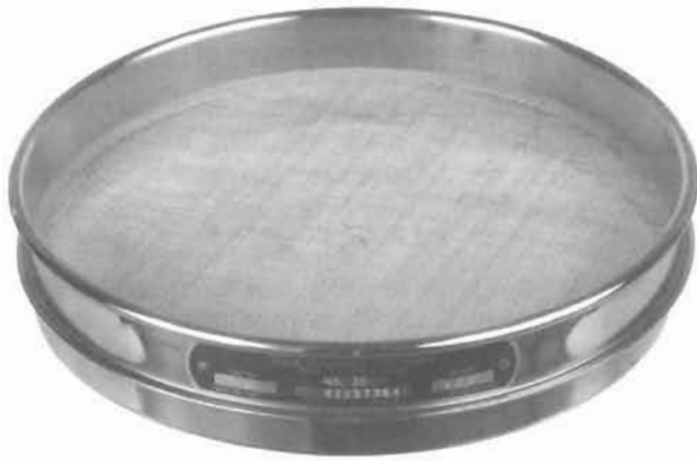
19-1 figure Fisher USA Standard test sieve. Range of mesh sizes is available for various particle size separations.
